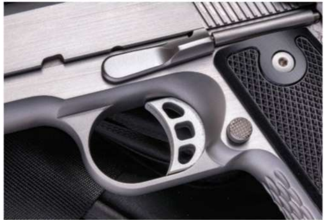
The serrated and curved aluminum trigger shoe is standard length. The trigger pull was tested at 3 pounds, 9 ounces. Within reach is the mag-release button and slide-lock/-release lever.
