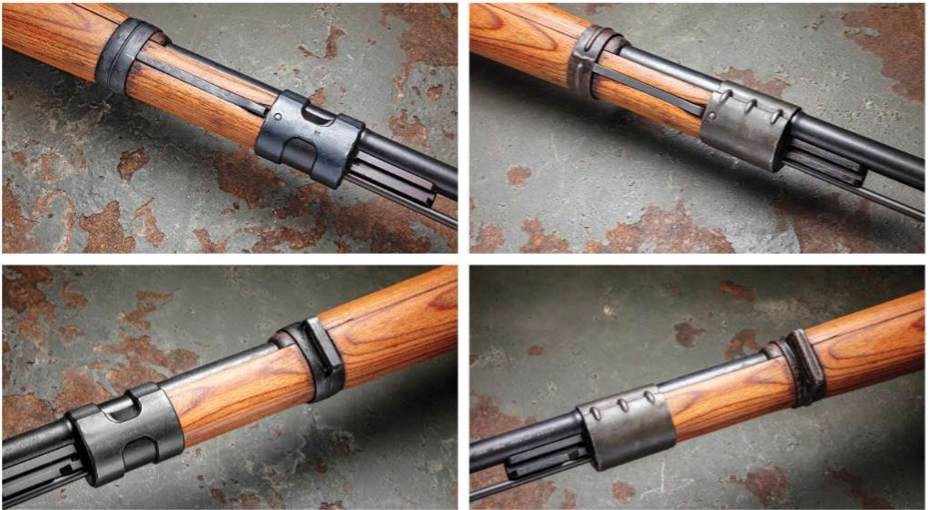
The Mitchell's Mausers receiver dates the K98k to 1944. The rear and "H"-type front bands (above, left) were incorrect. Due to war-time production issues, milled parts were depleted. The front and rear bands became stamped-and-welded parts (above, right).
