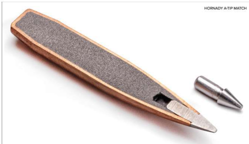
The aluminum tip of Hornady's A-Tip Match projectile is precision machined for reduced drag. The shaft is longer than polymer tips, shifting weight and stabilizing the bullet.
