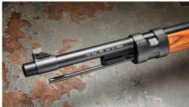
The Mitchell's Mausers receiver dates the K98k to 1944. The rear and "H"-type front bands (above, left) were incorrect. Due to war-time production issues, milled parts were depleted. The front and rear bands became stamped-and-welded parts (above, right).
