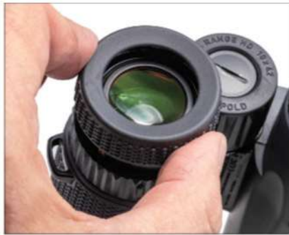
Eye relief measured 17mm. Both ocular lenses feature oversized eyepieces with finger-adjustable textured rubber eyecups. Counter-clockwise to extend, clockwise to collapse the distance, they are intuitive to rotate into position.
