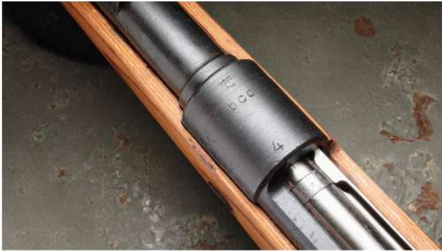
The "bcd" marking indicates that the receiver was manufactured by Gustloff-Werke. Above "bcd" is a Waffenampt stamp, a German inspection proofmark that also appears on the left-side of the receiver and barrel. The "4" denotes "1944" production.
