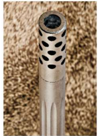
The radial ported muzzlebrake mitigates felt recoil. The barrel can be suppressed.
