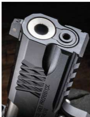
The stainless-steel bull barrel features an integral ramp for supporting the feeding of 9mm ammunition. The muzzle features a blended crown, protecting the 1-in-10-inch-twist rifled bore.
