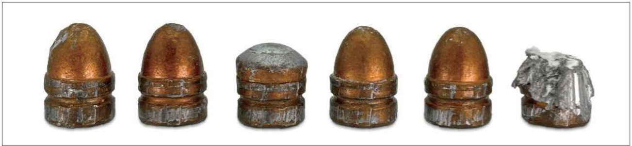
D&L Sports GSP 200-grain RNSWC bullets after barrier testing. From above, left: Bare gel; heavy clothing; steel; wallboard; plywood; and automobile safety glass. Note: Only the steel and glass barriers had any noticeable impact on the coated-lead projectiles.
