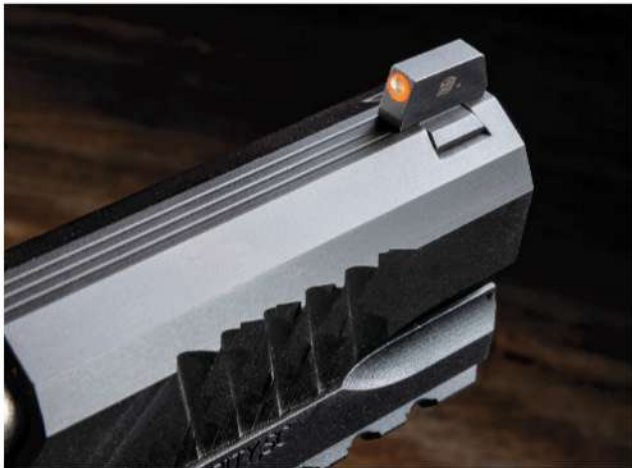
A three-line serrated topstrap leads to the dovetailed XS Sight, featuring an orange ring surrounding a tritium insert. The sight is suppressor compatible and will co-witness with most red-dot sights.
