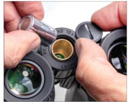
Remove the cap to change the CR2 battery. One battery powers approximately 3,000 uses of the rangefinder.
