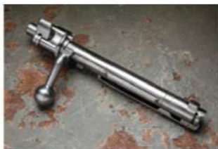
Mitchell's Mauser bolts were often polished (above, left), removing mismatched part numbers. The project's bolt was bead blasted and reblued, simulating late-war production quality.
