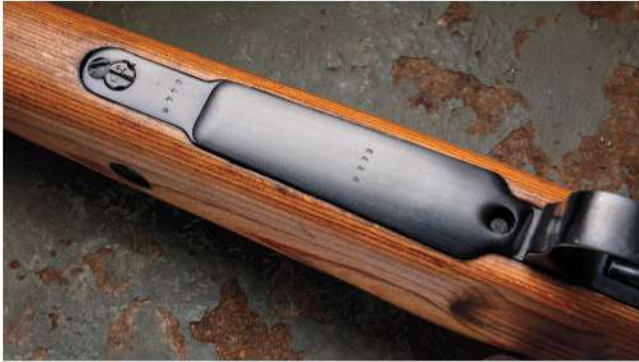
Mitchell's Mausers sanded and removed markings from components, including the rifle's bottom metal. They were remarked to match the last four digits of the receiver's serial number. The project rifle was corrected with a stamped "byf"-marked floorplate.
