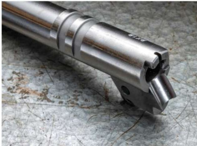
The stainless-steel bull barrel features an integral ramp for supporting the feeding of 9mm ammunition. The muzzle features a blended crown, protecting the 1-in-10-inch-twist rifled bore.
