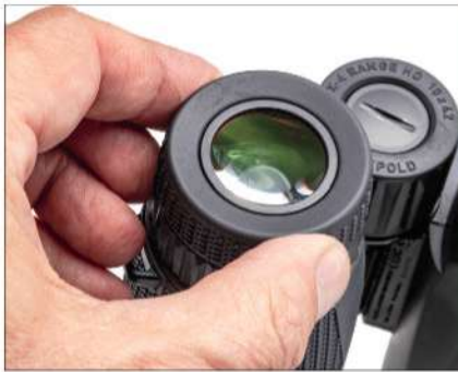
Eye relief measured 17mm. Both ocular lenses feature oversized eyepieces with finger-adjustable textured rubber eyecups. Counter-clockwise to extend, clockwise to collapse the distance, they are intuitive to rotate into position.
