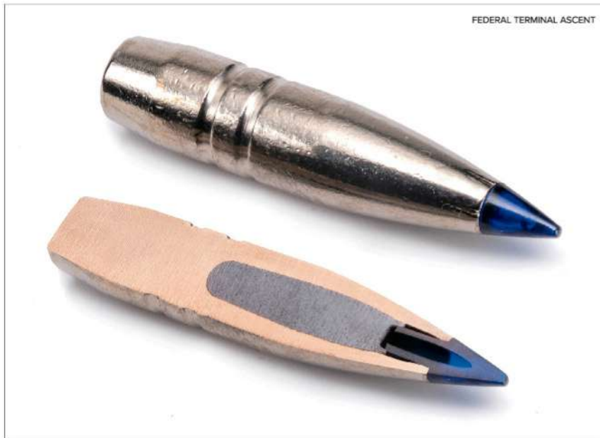
Terminal Ascent features Federal's Slipstream Tip with a hollow-core and AccuChannel Groove. The tip initiates expansion of the bonded, nickeled jacket and core.
