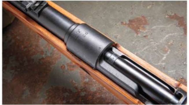
The "bcd" marking indicates that the receiver was manufactured by Gustloff-Werke. Above "bcd" is a Waffenampt stamp, a German inspection proofmark that also appears on the left-side of the receiver and barrel. The "4" denotes "1944" production.
