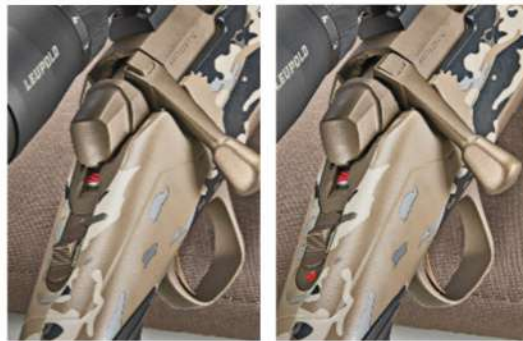
The bolt-unlock button rises when the tang safety is engaged (above, left). It's used to unload or inspect the chamber. Under the bolt shroud is the striker tab status.
