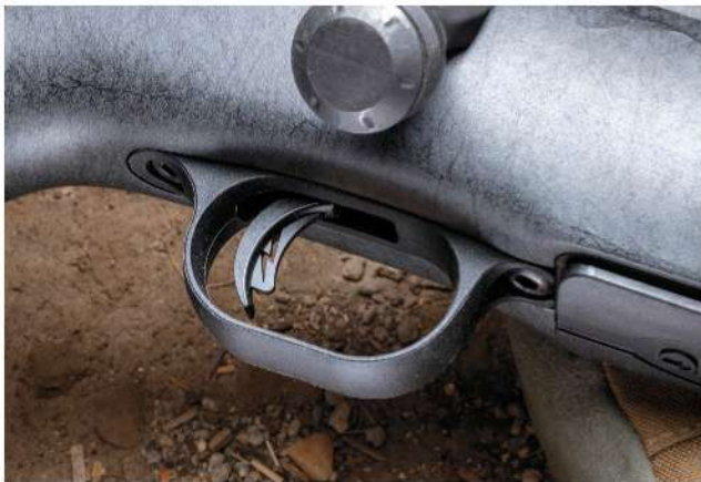
The Lighting Bolt Action (LBA) trigger is adjustable from 2 to 7 pounds. The safety blade with lightning bolt logo prevents the trigger from being manipulated unless the safety is pressed flush.
