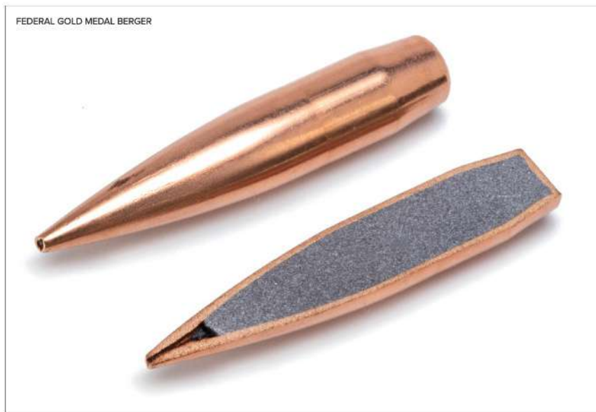
Gold Medal Berger is known for its high BC, and long-drawn copper jacket surrounding lead antimony. On impact, the open-tip design is crushed to initiate expansion.
