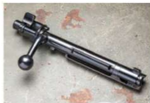
Mitchell's Mauser bolts were often polished (above, left), removing mismatched part numbers. The project's bolt was bead blasted and reblued, simulating late-war production quality.
