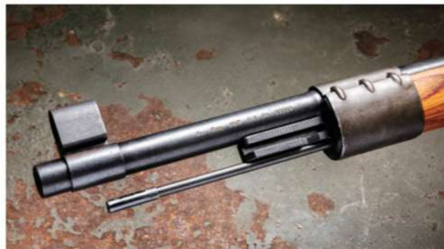
The Mitchell's Mausers import marks on the barrel were left intact to maintain this project's true history. However, in addition to correcting the front band, a steel sight hood was installed.
