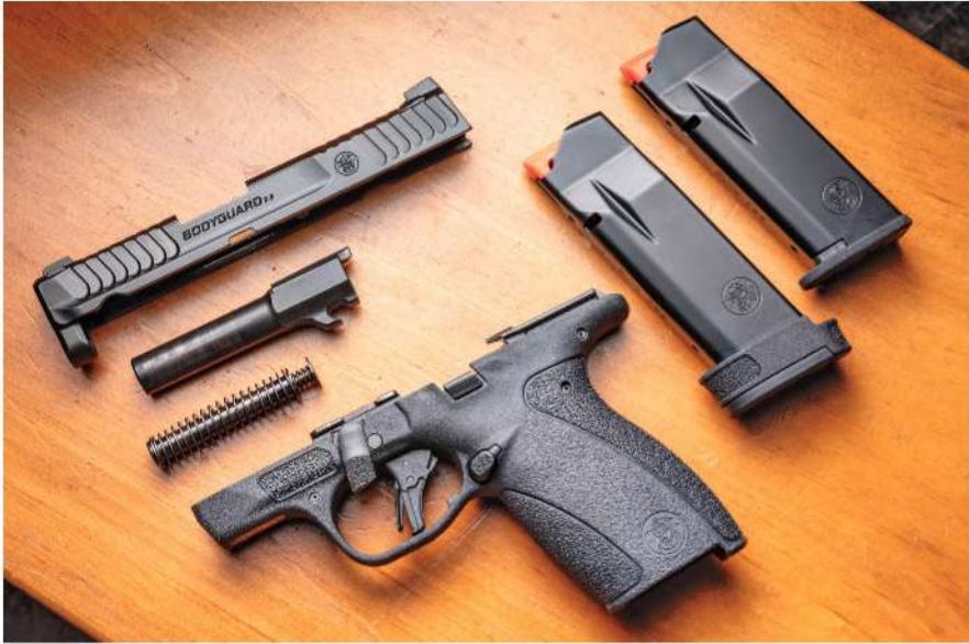
Disassembly and reassembly of the Bodyguard 2.0 is a familiar affair. With the magazine removed and slide locked back, the takedown lever rotates down for fieldstripping.
