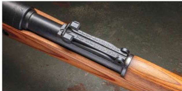
The rear sight was corrected with a replacement that lacked marks on the back side.
